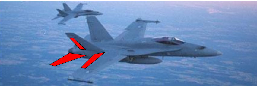
Figure 1. Areas under investigation for the moisture detection (port and starboard side of the aircraft). Red indicates the interest area of flight control surfaces (rudder, trailing edge flap and horizontal stabilizer). Courtesy of the FiAF.
